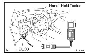
To check the DTCs, connect the OBD scan tool or hand-held tester to Data Link Connector 3 (DLC3) on the vehicle. The OBD scan tool or hand-held tester also enables you to erase the DTCs and check freezed frame data and various forms of engine data. (For operating instructions, see the OBD scan tool's instruction book.)
