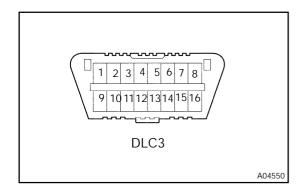
(2) Using SST, connect between terminals 13 (TC) and 4 (CG) of DLC3.
