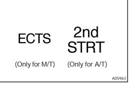
(3) Read the diagnostic trouble code from 2nd STRT indicator (only for A/T)/ETCS indicator (only for M/T) on the combination meter.
