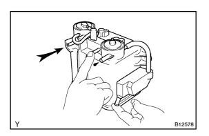
(2) While holding the ports B and D closed, blow air (1.76 kPa (18 gf/cm, 0.26 psi)) into the port A and check that air does not flows from the port D.
