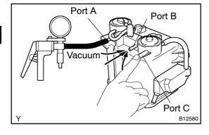
While holding the port C closed, apply vacuum (1.32 kPa ( 10 mmHg, 0.39 in.Hg)) to the port A and check that air flows into the port B.
