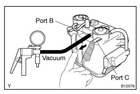
(3) Apply vacuum (3.43 kPa (26 gf/cm , 1.01 psi)) to port B, check that the vacuum does not decrease when port C is closed, and check that the vacuum decreases when port C is released.
