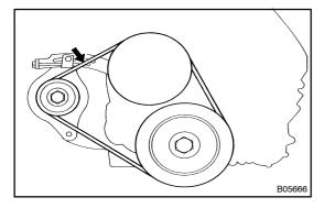
(b) Check the drive belt deflection by pressing on the belt at the points indicated in the illustration with 98 N ( 10 kgf, 22 lbf) of pressure.
