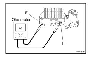
(b) Using an ohmmeter, check the continuity between terminals F and E.
