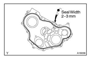
(b) Apply seal packing to the timing gear cover as shown in the illustration.
