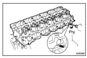
(c) Lift the cylinder head from the dowels on the cylinder block, and place the cylinder head on wooden blocks on a bench.
