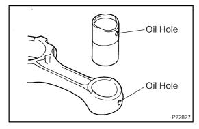
(4) Align the oil holes of t new bushing and the connecting rod.
