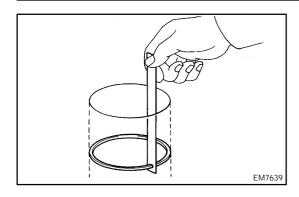
(3) Using a feeler gauge, measure the end gap.
