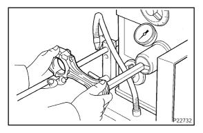
(6) Using a pin hole grinder, hone the busing to obtain the standard specified clearance (see item C above) between the busing and piston pin.
