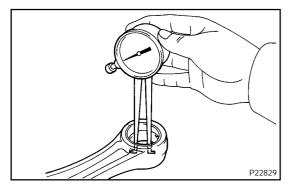
(c) Inspect piston pin oil clearance
