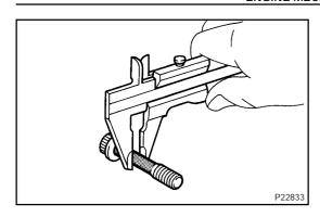
(b) Inspect connecting rod bolts Using vernier calipers, measure the tension portion diameter.
