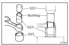
(5) Using SST and a press, press in the bushing. SST 09222-17011 (09222-05021, 09222-05031, 09222-05041)
