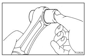
(7) Check the piston pin fit at normal room temperature. Coat the piston pin with engine oil, and push it into the connecting rod engine oil, and push it into the connecting rod with your thumb.
