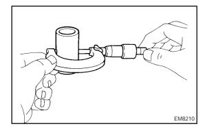
(2) Using micrometer, measure the piston pin diameter. **Piston pin diameter**:
