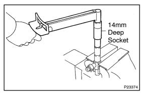
(b) Using a 14 mm deep socket wrench, torque the retaining nut.
