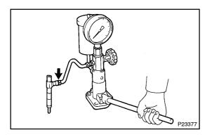
(c) Install the injection nozzle to the injection nozzle hand tester and bleed air from the union nut.
