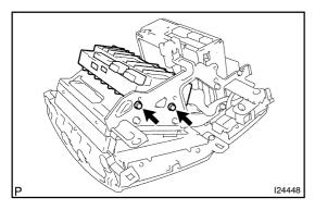
(c) Remove the 2 screws and A/C amplifier.
