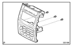
(c) Remove 3 screws and integration control panel.
