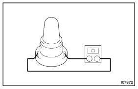
(c) Apply the tester as shown in the illustration to the test for continuity.
