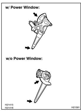
At the time of assembly, apply MP grease to the window regulator.
