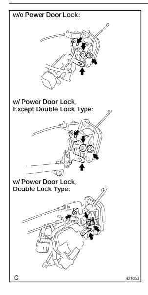
S Remove the protector, and apply MP grease to the sliding and rotating parts of the door lock.
