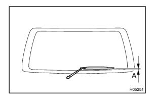
(d) Adjust the installation position of the wiper arms to the position shown in the illustration.
