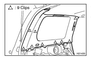
**8. INSTALL UPPER ROOF SIDE INNER GARNISH** Install the upper roof side inner garnish with the clip.
