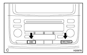
(b) Turn the ignition switch to ACC as pressing the "SEEK UP" and "DISC" switches at the same time.
