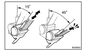
(d) Make sure that the belt can be pulled out at a tilt of 15 degrees or less, and cannot be pulled out over 45 degrees of tilt.
