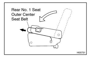
(d) When folding down the seatback forward and extracting the seat belt slowly, check that the belt is locked after a certain length (approx. 500 mm (19.69 in.)) of the belt has been extracted.
