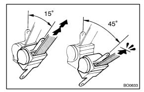
(g) Make sure that the belt can be pulled out at a tilt of 15 degrees or less, and cannot be pulled out at over 45 degrees of tilt.
