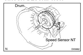
The speed sensor NT detects the rotation speed of the input shaft from the rotation of the drum. Its construction is the same as that of the speed sensor SP2.
