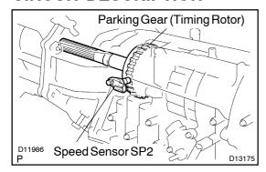
The speed sensor SP2 detects the rotation speed of the transmission output shaft and sends signals to the Engine and ECT ECU. The Engine and ECT ECU determines the vehicle speed based on these signals. An AC voltage is generated in the speed sensor SP2 coil as the parking gear mounted on the rear planetary gear assy rotates, and this voltage is sent to the Engine and ECT ECU. The parking gear on the rear planetary gear is used as the timing rotor for this sensor.
