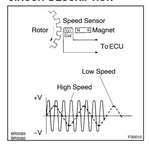
The speed sensor detects wheel speed and sends the appropriate signals to the ECU. These signals are used for control of both the ABS & BA & TRC & VSC control system. The front and rear rotors each have 48 serrations.
