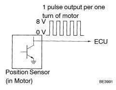
The position sensor senses movement of the seat and send pulse signals to the ECU. The position sensor sends pulse to the ECU in proportion to the amount of seat movement, as shown in the diagram on the left.
