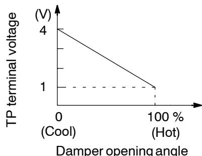
This sensor detects the position of the front air mix damper and sends the appropriate signals to the A/C amplifier.
