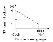
This sensor detects the position of the rear air mix damper and sends the appropriate signals to the rear A/C amplifier.
