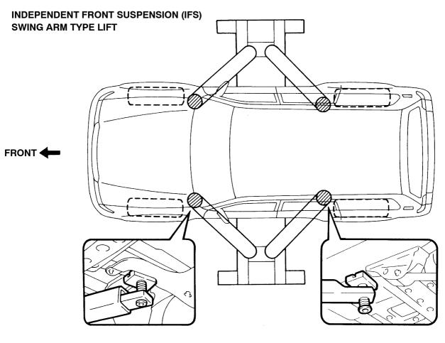
NOTICE: When lifting the vehicle, place the supports correctly at the positions shown above.
