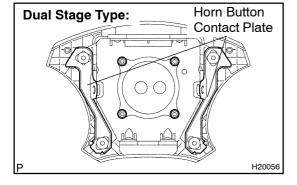
• Check the deformation of the horn button contact plate on the steering wheel pad (with airbag).
