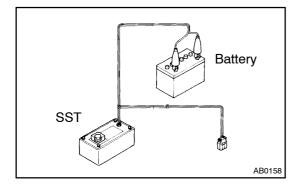
(1) Connect the red clip of the SST to the battery positive (+) terminal and the black clip to the battery negative (-) terminal.
