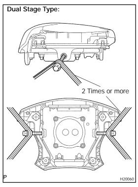
(4) Using 3 wire harness, wind the wire harness at least 2 times each around the bolts installed on the left and right sides of the steering wheel pad.
