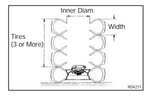
S Covering method using tires: Place at least 3 tires with no disc wheels on top of the tire with disc wheel to which the steering wheel pad is tied.
