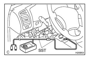
(7) Connect the connector of SST to the airbag connector of the spiral cable.
