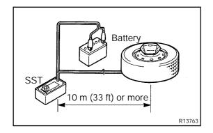
(2) Move the SST at least 10 m (33 ft) away from the steering wheel pad tied down on the disc wheel.
