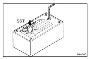
(2) Press the SST activation switch, and check that the LED of the SST activation switch comes on.
