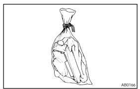
(g) Dispose of the steering wheel pad (with airbag).
