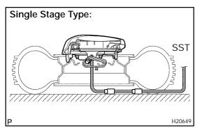
(5) Face the upper surface of the steering wheel pad upward. Separately tie the left and right sides of the steering wheel pad to the disc wheel through the hub nut holes. Position the steering wheel pad connector so that it hangs downward through a hub hole in the disc wheel.
