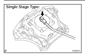
(3) Single stage type: Connect the connectors of the SST to the steering wheel pad connector.
