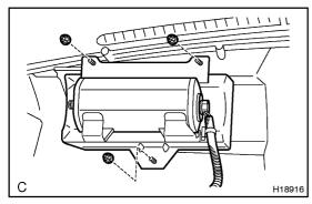
7. REMOVE FRONT PASSENGER AIRBAG ASSEMBLY Remove the 3 nuts, then remove the front passenger airbag assembly.
