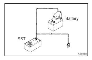
(c) Check the functioning of the SST (See step 1–(a) on page RS–20). SST 09082–00700
