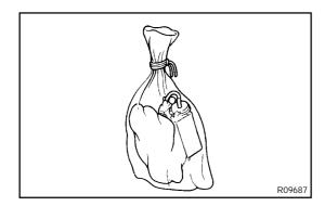
3. DEPLOYMENT WHEN-DISPOSING OF FRONT PAS-SENGER AIRBAG ASSEMBLY DEPLOYED IN A COL-LISION
