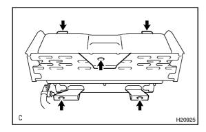
(1) While passing the wire harness through the installation holes indicated by arrows in the illustration, wind the wire harness around the tire.
