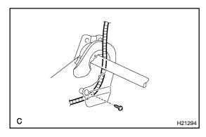
(e) Remove the 2 screws and RH reclining adjuster inside shield, then disconnect the side airbag connector.
