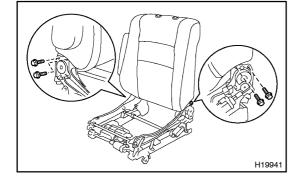
(d) Remove the 4 bolts and seatback assembly.
