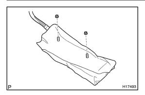
(1) Install the 2 nuts to the side airbag assembly.
