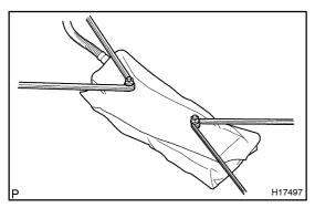
(2) Wind the wire harness around the stud bolts of the side airbag assembly as shown in the illustration.
