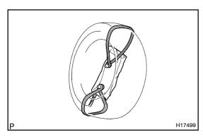
(3) Position the side airbag assembly inside the tire with the airbag deployment direction facing inside.
