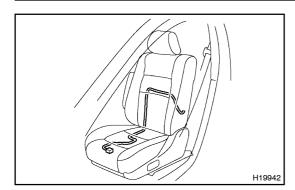
(b) Disconnect the side airbag connector.
