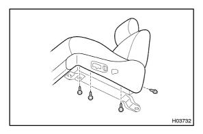
(b) Install the seat cushion outer shield with the 4 screws.
