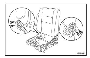
(b) Install the seatback assembly with the 4 bolts.
