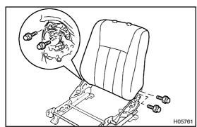
(b) Install the seatback assembly with 4 bolts.
