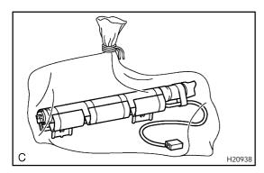
3. DEPLOYMENT WHEN DISPOSING OF CURTAIN SHIELD AIRBAG ASSEMBLY WITH AIRBAG DEPLOYED IN COLLISION
