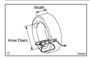
(2) Position the curtain shield airbag assembly inside the tire with the airbag deployment direction facing inside.
