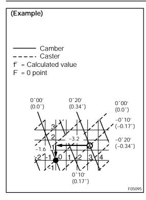
(c) How to read adjustment chart (using examples).
