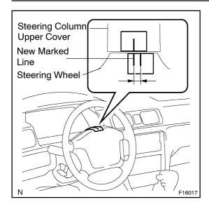
(d) Turn the steering wheel to its straight position.
