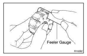
(b) Using a feeler gauge, measure the clearance between the rotor groove and plate.
