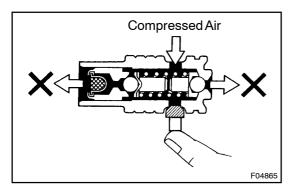
(b) Check the flow control valve for leakage. Close one of the holes and apply compressed air 392 - 490 kPa (4 - 5 kgf/cm², 5 7 - 71 psi) into the opposite side hole, and confirm that air does not come out from the end holes.
