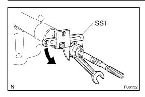
(b) Using a spanner to hold the steering rack steady, and using SST, remove the rack end.
