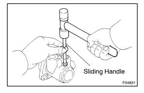
Using plastic hammer and sliding handle, lightly tap in a new seat.
