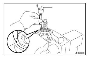
(f) Using a punch, stake the nut.
