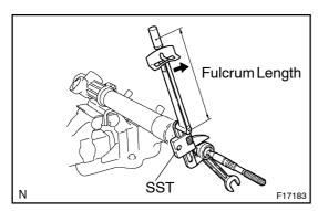
(b) Using a spanner to hold the steering rack steady, and using SST, torque the rack end.
