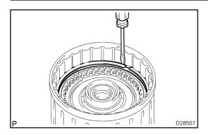
(b) Using a screwdriver, install the 2 hole snap rings on the clutch drum sub assy.
