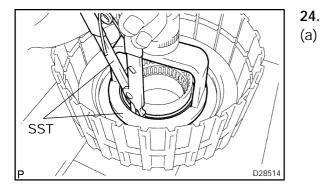
(a) Place SST on the direct clutch piston, and compress the return spring with a press.
