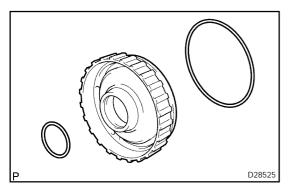
(b) Remove the 2 O-rings from the forward clutch piston.
