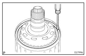
(b) Using a screwdriver, install the snap ring on the clutch drum and the input shaft assy.
