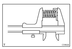
25. INSPECT DIRECT CLUTCH RETURN SPRING SUB-ASSY
