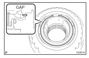
(d) Set the end gap of the snap ring in the piston as shown in the illustration.
