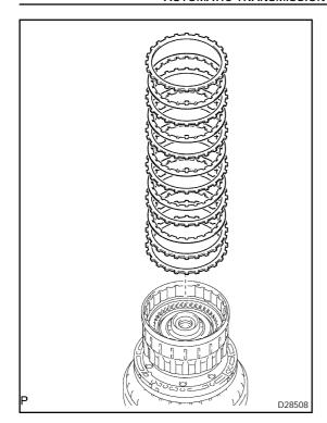
(b) Remove the reverse clutch flange, the 6 plates and the 5 discs from the clutch drum assy.
