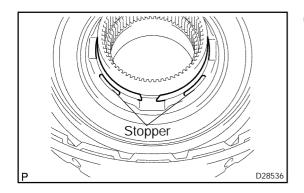
(g) Set the end gap of the snap ring in the piston as shown in the illustration.
