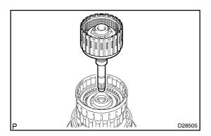
Remove the input shaft assy from the clutch drum assy. (b)
