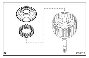
(b) Remove the clutch balancer No.1 and the forwerd clutch return spring from the inputshaft assy.
