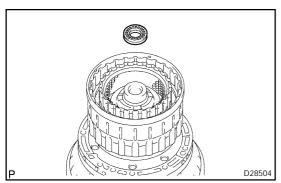
(b) Install the thrust needle roller bearing to the clutch drum
