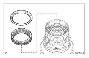
(b) Remove the reverse clutch reaction sleeve, the clutch cushion plate, the reverse clutch flange, the 5 reverse clutch discs, and the 4 clutch plates from the reverse clutch hub sub assy.
