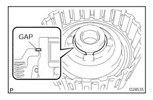
(f) Set the end gap of the snap ring in the piston as shown in the illustration.
