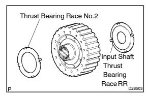
(b) Remove the thrust bearing race No.2 and the input shaft thrust bearing race RR from the multiple disc clutch clutch hub.
