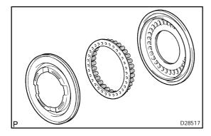
(b) Install the clutch balancer No.2 and the direct clutch return spring to the direct clutch piston sub assy.
