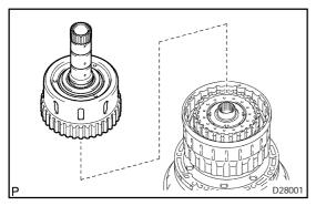
(b) Install the forward clutch hub sub assy to the clutch drum assy.
