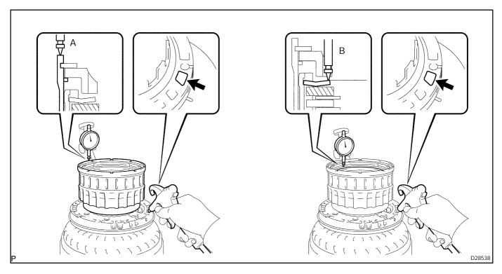
(b) If the pack clearance is outside the standard, select & install a clutch flange that makes the pack clearance to be within the standard.
