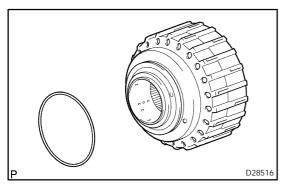
(c) Remove the O-ring from the clutch drum.
