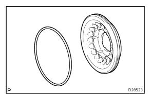
(c) Remove the O-ring from the clutch balancer No.1.
