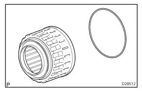
(b) Remove the O-ring from the reverse clutch piston sub assy.
