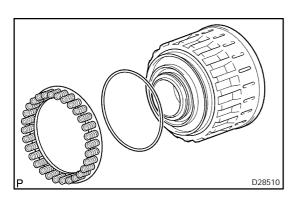
28. INSTALL REVERSE CLUTCH RETURN SPRING SUB-ASSY
