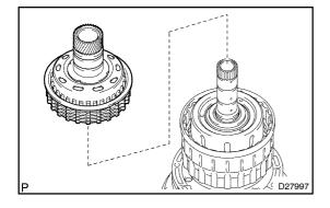
Remove the reverse clutch hub sub assy, the reverse clutch reaction sleeve, the clutch cushion, the plate reverse clutch flange, the 5 reverse clutch discs, and the 4 clutch plates from the clutch drum assy.
